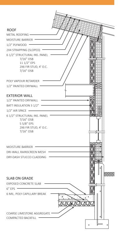
Wall Section: Common assemblies and details found in this structure. Note the use of SIPs to allow for thinner walls with adequate insulation. The water barrier system reduces risk of deredation through rainscreen cladding. A lack of insulation in the concrete slab on grade and direct connection to the wall results in some thermal bridging.
