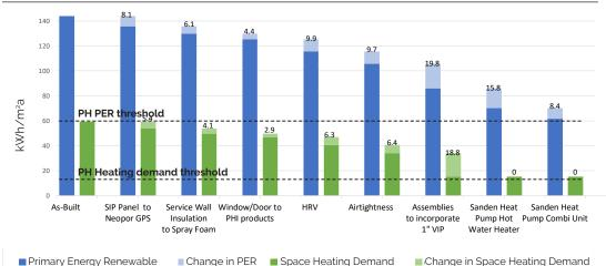
Due to the building's relatively small size, its form factor is 4.83, whereas that of a typical Passive House single-family house is around 3.
