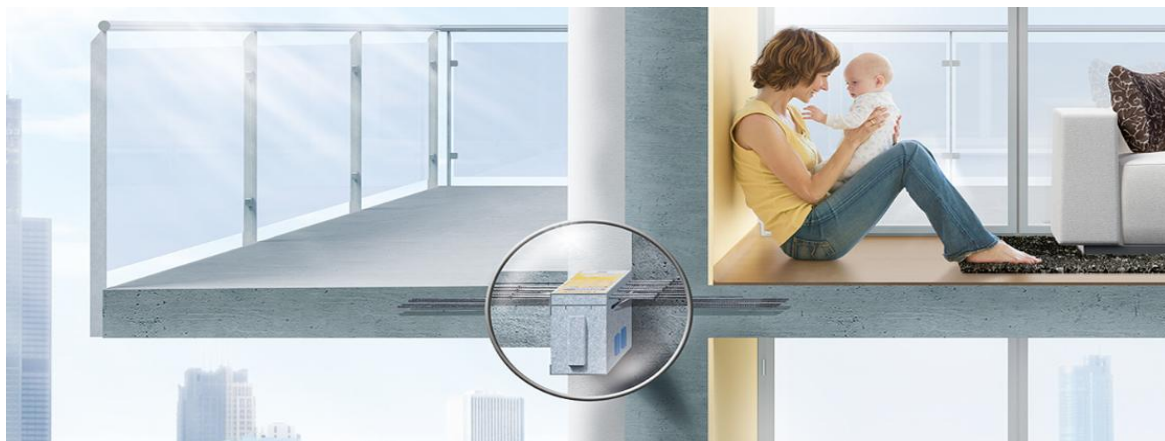
Figure 20: Load-bearing thermal-break element preventing cold-bridging from exposed balcony slab into apartment © Schöck
