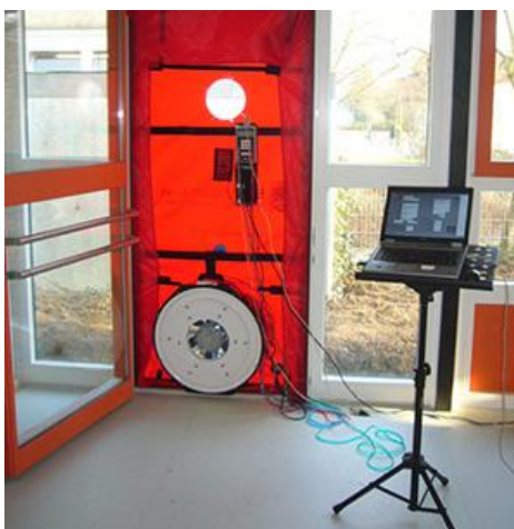
Figure 26: Air permeability testing using a typical blower door rig
