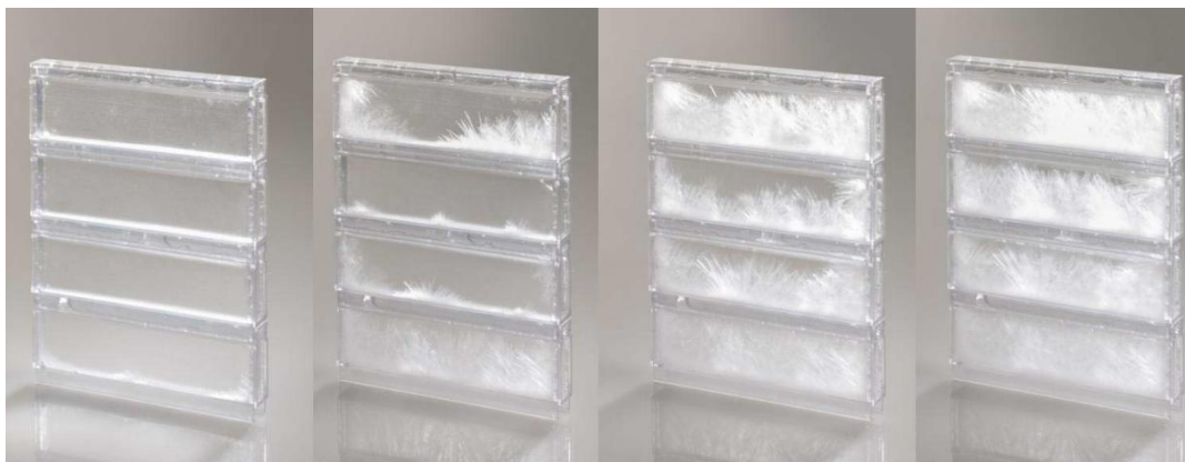
Figure 18: PCM salts embedded within glazing change translucency during phase-change whilst absorbing significant thermal loads © CrystalX
