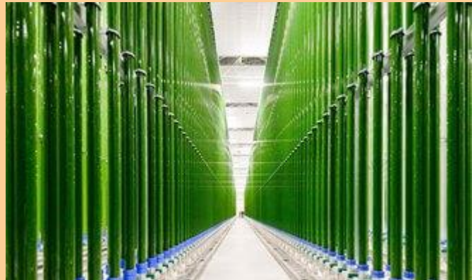
Figure 2.19: Picture of in-pipe algae growth system (from https://www.ecoduna.com/en/company/our-usp/ )
