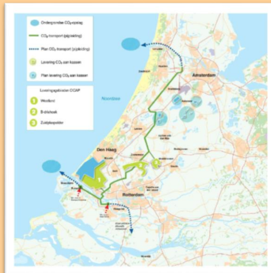
Figure 2.12: OCAP CO 2 pipeline system in Rotterdam, The Netherlands. Source: ocap.nl
