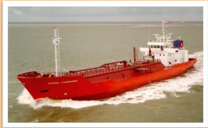
Figure 2.14: Picture of CO 2 transportation vessel (from https://www.antonvveder.com/fleet/coral-carbonic )
